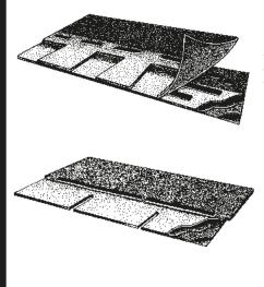
Laminated shingles consist of two or more layers bonded together, giving them added dimension for a shake-like appearance.
