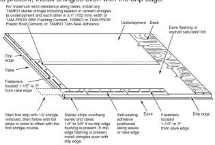
SHINGLE APPLICATION: Start the first course with a full size shingle and overhang the rake edge 1/4 in. if drip edge is not present. If drip edge is present, align shingle edge with drip edge flashing. Cut 10-3/8 in. from a full shingle to form a shingle 29 in. long. Use this to start the second course (see diagram below). Cut a 23 in. long shingle to start the third course. Use the remaining 16-3/8 in. piece
