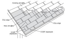
First Course: Remove an amount from the butt edge of a full-size shingle so that the remaining portion of the shingle fits between the butts of the existing third course. This course must also be applied evenly along the eaves edge of the new starter strip.
